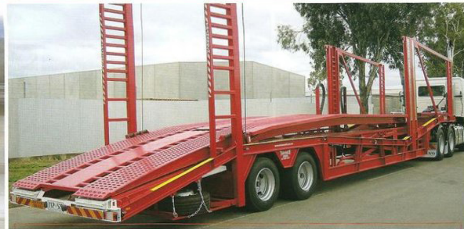
The whole deck on this unique Transmech car carrier lowers to provide a level-loading platform. Having this feature makes the task of securing the car not only safer, but faster. Once loaded the whole deck can be positioned in any way to suit the load.
